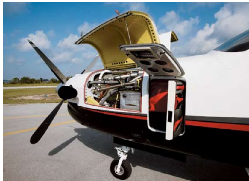
■ The crew door has become a popular option, even though it adds $75,000 to the price. The main cabin door is extremely large and has an electrically powered system that pulls it closed, ready for latching. The cowling opens quickly for access to the PT6 turboprop engine. In the lower photo you can see two bleed air lines running along the engine, the only visible change under the cowling.
