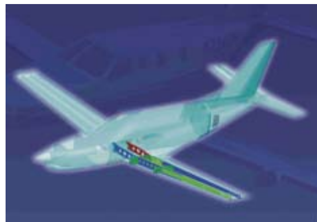
Fail-safe Spar Design
